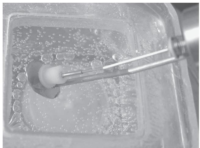
Fig. 1. A photo of a measurement of trap thickness changes in *Utricularia reflexa* using a linear position sensor. The trap is fixed in the sensor laterally.
