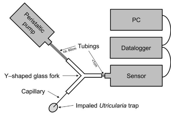
Fig. 1. Schematic drawing of the experimental setup used for the CNP measurements. Note that length ratios are not correct.
